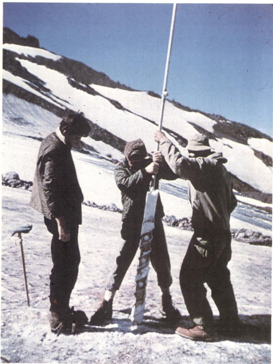
The SEARCH team decides to bore through the glacial ice pack with a hand drill in hopes of hitting pieces of wood with the bit. With extension poles it was possible to bore 35 feet into the ice pack.
